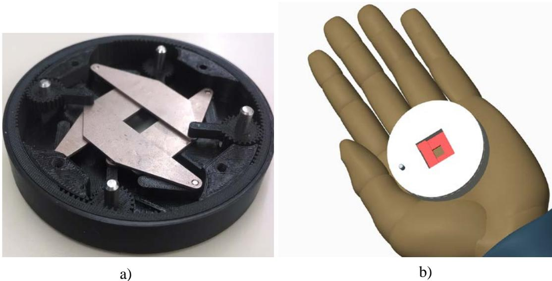
Figure 17: a) rapid prototyped SBIORT collimator, b) CAD model of SBIORT collimator's size with respects to a hand
